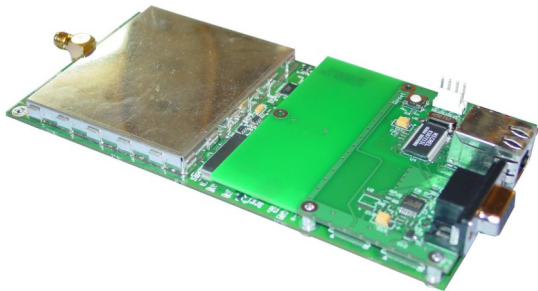
Tiamis-800 transceiver with Option 1200 - interface board
