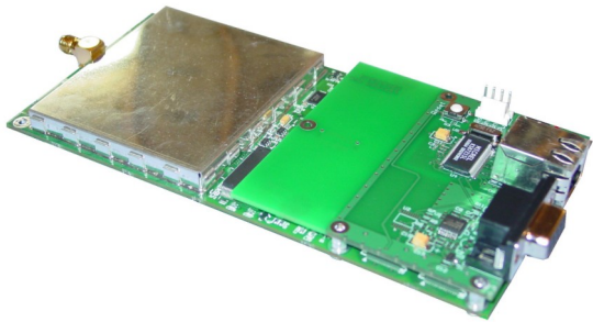
Tiamis-800 transceiver with Option 1108 - interface board
