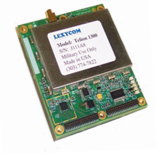
Telion-1300 fully digital, spread spectrum software defined radio, board level
