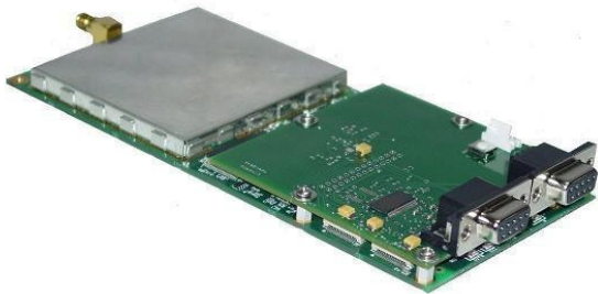
Tiamis-800 transceiver with Option 1103 - interface board
