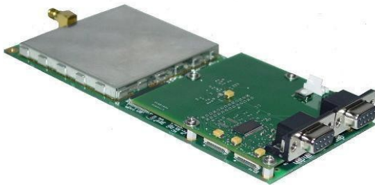
Tiamis-800 transceiver with Option 1100 - interface board
