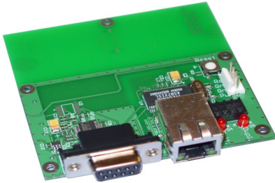
Option 1200 - Ethernet and diagnostics port interface board
