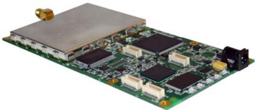
Board level Tiamis-800 software defined radio transceiver
