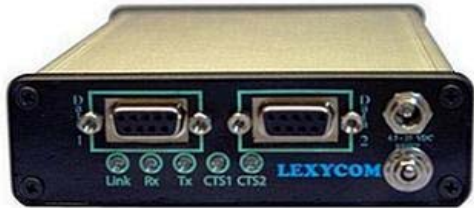
Tiamis-800, software defined radio transceiver, extruded aluminum enclosure
